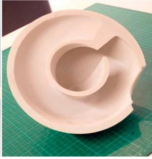
This is the reason why the Hylixa has to be 3D printed. This bowl-shaped disc is a cross-section of the elaborate helical transmission line design; a shape that cannot be created by any other means.
