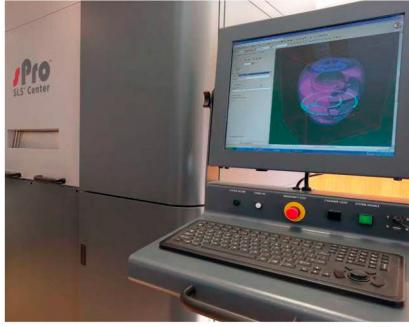
The enclosure of the Node Audio Hylixa uses an industrial-grade Selective Laser Sintering (SLS) process. A three-dimensional model of the enclosure is uploaded to a computer that runs what's known as a 'slicer' program. This divides the three-dimensional file into two-dimensional layers, which are overlaid to build up the full enclosure. This takes hours!
