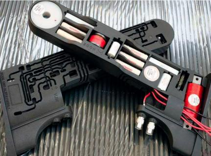
This is the point where other loudspeaker makers get a bit jealous. The whole crossover network is built into a magazine that slots into the loudspeaker stand itself. It has been carefully created to act as housing for the high-grade components in that crossover, in the form of a 3D puzzle, albeit one that uses high-grade cables, instead of etched tracks on a 2D circuit board.
