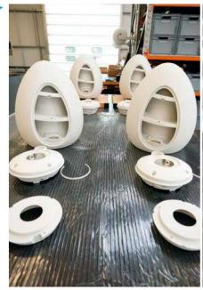
These are the component SLS-made parts needed to create the helical transmission line, the front baffle and its rear vent that feeds into the transmission line itself.
